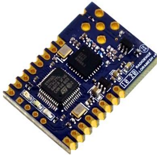
Figura 5 – Módulo LoRaWAN com Chirp Spread Spectrum
