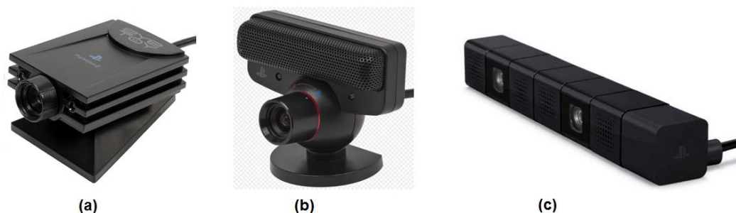
Figura 20 – Sensores de câmeras do Playstation. (a) EyeToy (PS2), (b) Eye (PS3), (c) Eye (PS4).
