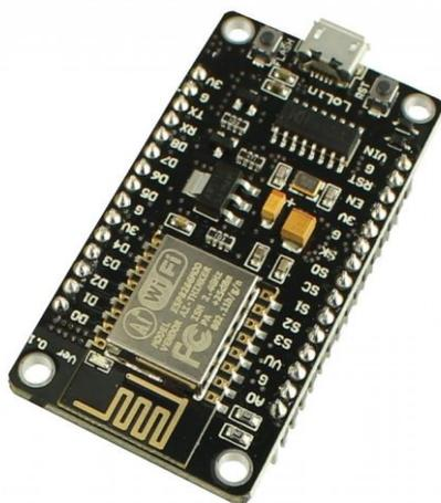
Figura (2) ESP8266 NodeMCU V3
