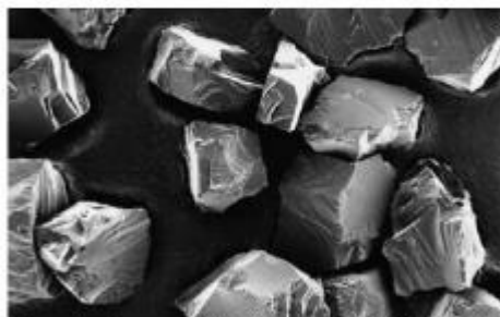
Sharp edges of monocrystalline diamonds of MetaDP ® Diamond Paste ensure clean and efficient cutting action.
