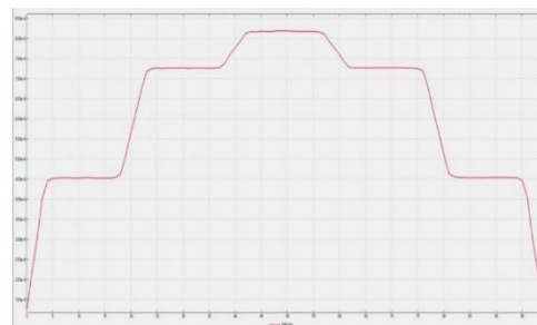
Fig. 2. Pressure Field as a Function of Position along the Axis between One End and the Other of the Resonant Cavity Vacuum System.
