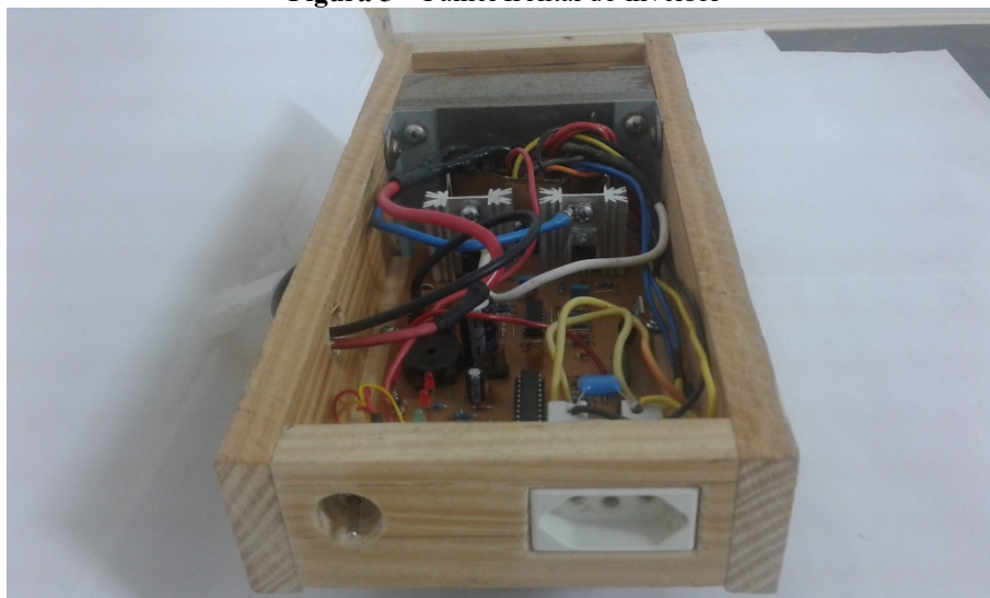
Figura 5 – Painel frontal do inversor
