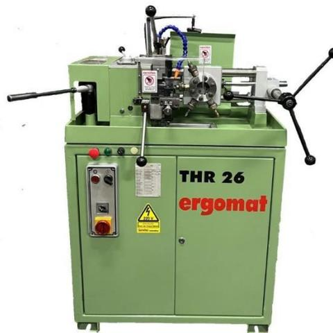
Figura 11 – Torno revolver
