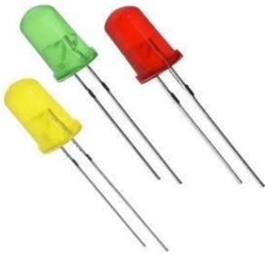
*Figura 11 Leds 5mm*
